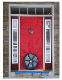
Newport Ventures recently completed a blower door test for a New York builder who had never before conducted the test on a home. Because the New York energy code will soon require blower door testing and limits on air leakage rates, this particular builder was interested to know where he stood with regards to these upcoming requirements.
