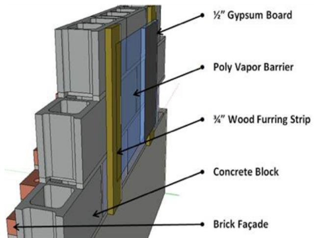
Figure 2. Exterior wall section showing limited depth furring and poly layer on inside face of concrete masonry units (CMU). Adding interior insulation board would have created a cold surface at this poly layer where moisture-laden indoor air leakage would condense.
