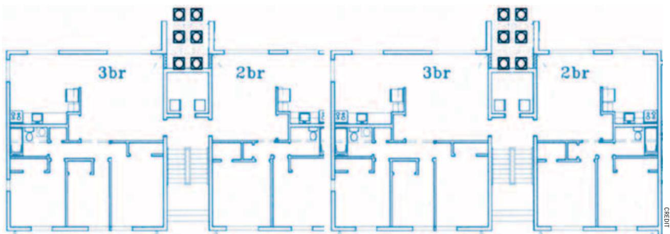
Figure 1. Floor plans for the 2- and 3-bedroom dwellings. Note separate HVAC closet.
