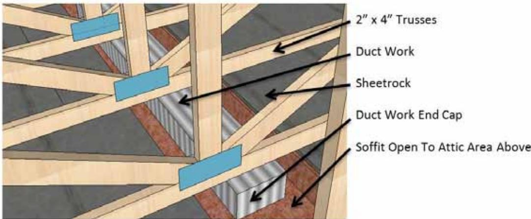
Figure 3. Diagram of duct bulkhead open to the attic space.
